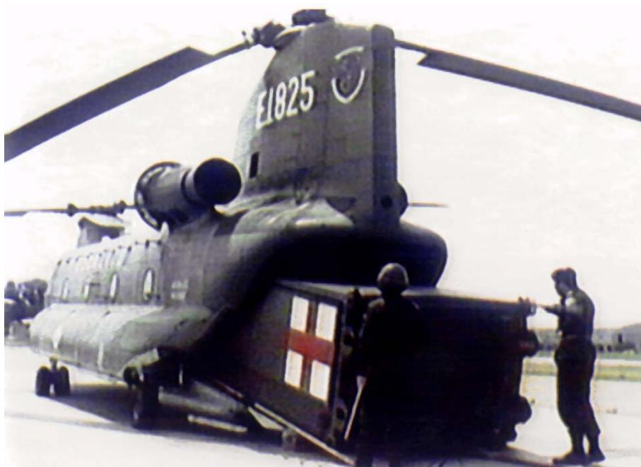
Each shelter and trailer is provided with a base structure and a set of teflon rollers for use during loading and unloading from helicopters. There are similar rollers at the ends of the hydraulic stabilizer jacks, so that both the shelters and the trailers can be moved sideways, for lining up in the operational stage.
