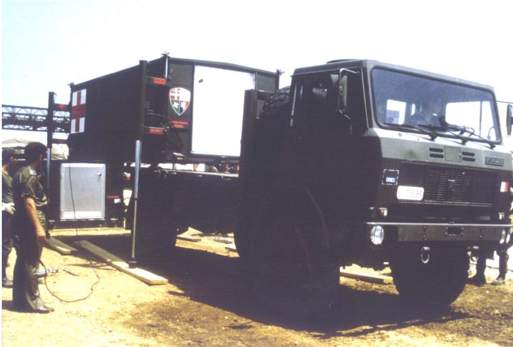
Each shelter and each trailer is provided with 4 stabilizer jacks, adjustable from inside and outside, with dual extension and dual effect and locking valves and an excursion of about 1600 mm.
